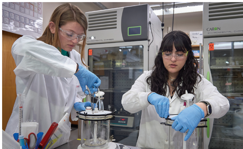
Researchers, Kylie Bodle, left, and Ghazal Vahidi, work with a biofilm reactor used to replicate real-world conditions. Kelly Gorham
