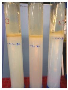
**Figure 1.** Experimental samples with a visible "crust" at the interface between the gel and the liquid.
