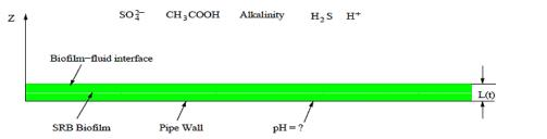
The model provides a theoretical framework for establishing a quantitative relationship between SRB activity and concentration of chemical species in biofilms that might affect corrosion processes in oilfield pipelines and other natural and industrially relevant environments.
