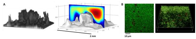
**Figure 2: (A)** Biofilm structure for measurement of deformation and CFD simulations. 3-d experimental structure from OCT imaging (left) in the computational model (right). **(B)** CLSM images of *Pseudomonas aeruginosa* (green) and biofilm-embedded 2 μm-microbeads (red), for determination of mechanical properties using microparticle actuation.
