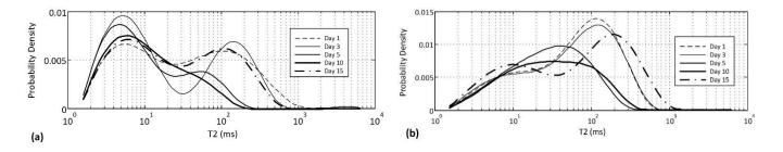
**Figure 1.**  $T_2$  distribution for ~275kHz well (a) and ~400kHz well (b) at inoculation (short dash line), during biofilm growth (solid lines), and after flushing and bleaching each well (dash-dot lines).
