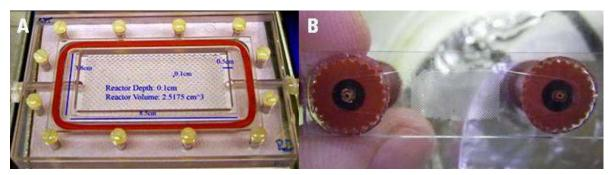
**Figure 1** - (A) 2D porous media reactor with 1mm pore structures. (B) 2D porous media reactor with  $100\mu$ m pore structures designed for CSLM imaging.
