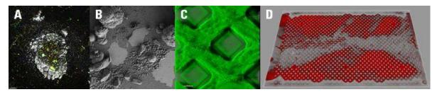
**Figure 2** – (A) CSLM image of a microbially induced  $CaCO_3$  crystal (gray) with cells attached (green and red). (B) FEM micrograph of microbially induced  $CaCO_3$  precipitation. (C) Living bacterial biofilm grown in a porous media reactor with 100µm pore structures. The bacterial strain is expressing green fluorescent protein, so no staining was required. (D) 3D CSLM reconstruction of a stained bacterial biofilm grown in the reactor pictured in Fig 1B.
