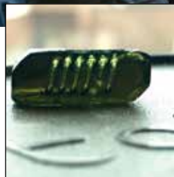
Right: Photo courtesy of Aaron Benjamin, undergraduate student at MSU This hydrogel cube, created by Aaron Benjamin using a 3D printer, is the consistency of Jell-O and contains internal channels for transporting liquids in and out of the cube.
