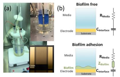
**Figure 1.** Impedance microbiology test apparatus (a) at the CBE to detect *in situ* biofilm growth in aqueous environments. Biofilm growth is detected through electrical modeling of sensor response (b).
